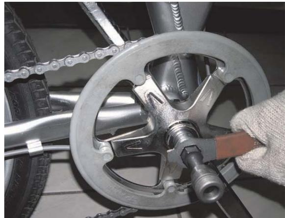
3. Check your frame for mounting space. The distance between the back of the bottom bracket and the rear tire should be at least 3.25" (82mm) for easiest mounting. If the distance is less than 3.25" you may need to fabricate special spacers or a custom mounting bracket.
