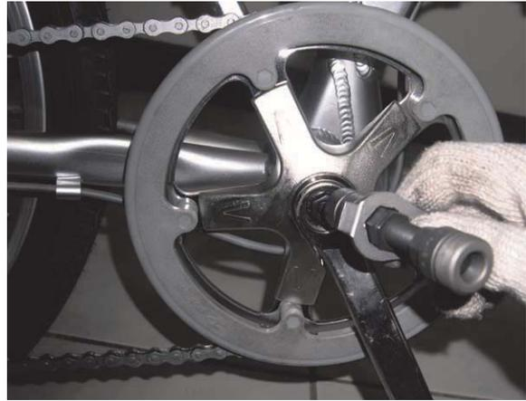
2. Use the crank removal tool to pull off both crank arms and chainwheel.
